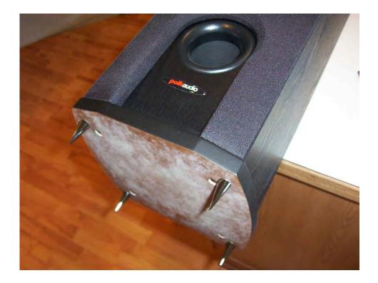
When placing speaker on carpet I recommend finding the spot were you want the speaker and then apply weight to the top of the speaker until the spikes pierce through the carpet and pad until they reach the subfloor.
